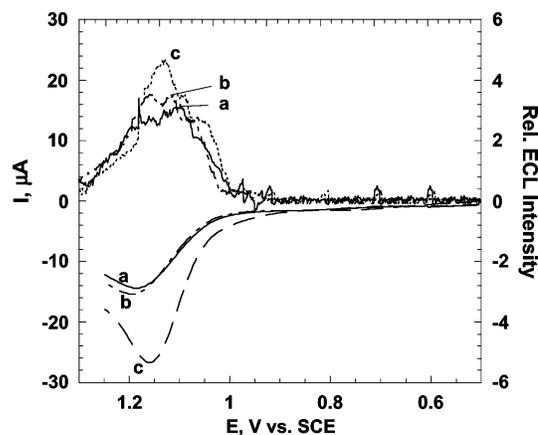
**Figure 7.** SWV and ECL response for (Ru-PVP/poly[G])<sub>2</sub> films on PG electrodes in pH 5.5 buffer + 50 mM NaCl: (a) no incubation; (b) incubated with saturated toluene control for 10 min.; (c) incubated with saturated styrene oxide for 10 min.
