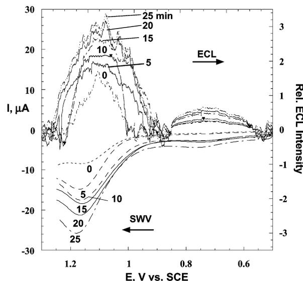
**Figure 5.** SWV and ECL responses for (Ru-PVP/ds-CT DNA)<sub>2</sub> films on PG electrodes in pH 5.5 buffer + 50 mM NaCl after incubations 37 °C with saturated styrene oxide. Numerical labels are incubation times in minutes.
