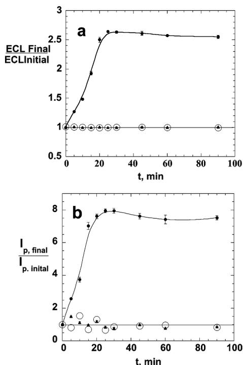
**Figure 6.** Influence of incubation time with styrene oxide (●), toluene (▲), and buffer alone (○) on (a) average ECL signals and (b) average SWV catalytic peak currents (final response/initial response) for (Ru/ds-CT DNA)<sub>2</sub> films. Error bars represent standard deviations for three trials, with 1 electrode/trial.
