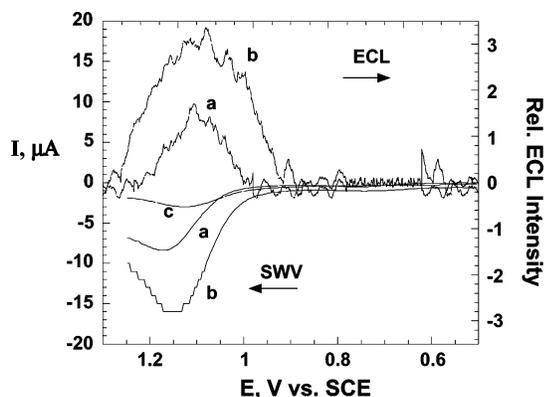
**Figure 4.** SWV and ECL for (a) (Ru-PVP/ds-CT DNA)<sub>2</sub> films and (b) (Ru-PVP/ss-CT DNA)<sub>2</sub> films on PG electrodes in pH 5.5 buffer + 50 mM NaCl and (c) SWV only for Ru-PVP film with no DNA.
