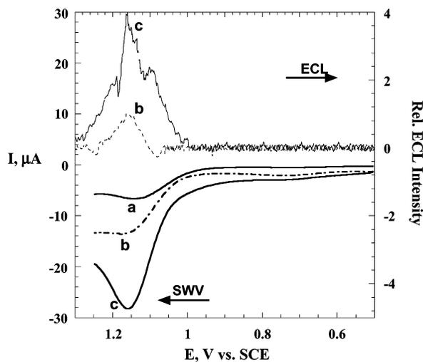
**Figure 3.** SWV and ECL response for (a) Ru-PVP, (b) (Ru-PVP/poly[G])/poly[C]<sub>2</sub> and (c) (Ru-PVP/poly[G])<sub>2</sub> films on PG electrodes in pH 5.5 buffer + 50 mM NaCl.
