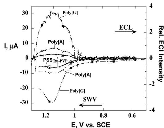
**Figure 2.** SWV and ECL response for films containing Ru–PVP on PG electrodes in pH 5.5 buffer + 50 mM NaCl. Films are Ru–PVP alone (○), (Ru–PVP/PSS)<sub>2</sub> (▲), (Ru–PVP/poly[A])<sub>2</sub> (◇), and (Ru–PVP/poly[G])<sub>2</sub> (■). Symbols are for curve identification only.
