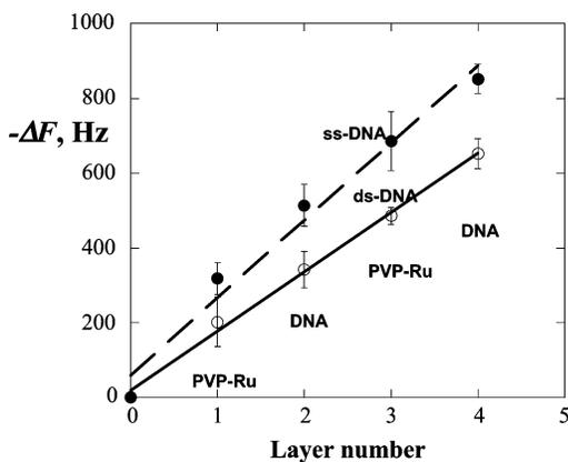
**Figure 1.** QCM frequency shifts for cycles of alternate PVP–Ru and CT-DNA layers on gold-quartz resonators coated first with mixed monolayers of mercaptopropionic acid/mercaptoethanol for ss-DNA (●) and ds-DNA (○) (average values for 3 replicate films).
